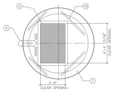
WET WELL PLAN VIEW @ GRADE LIFT STATION
