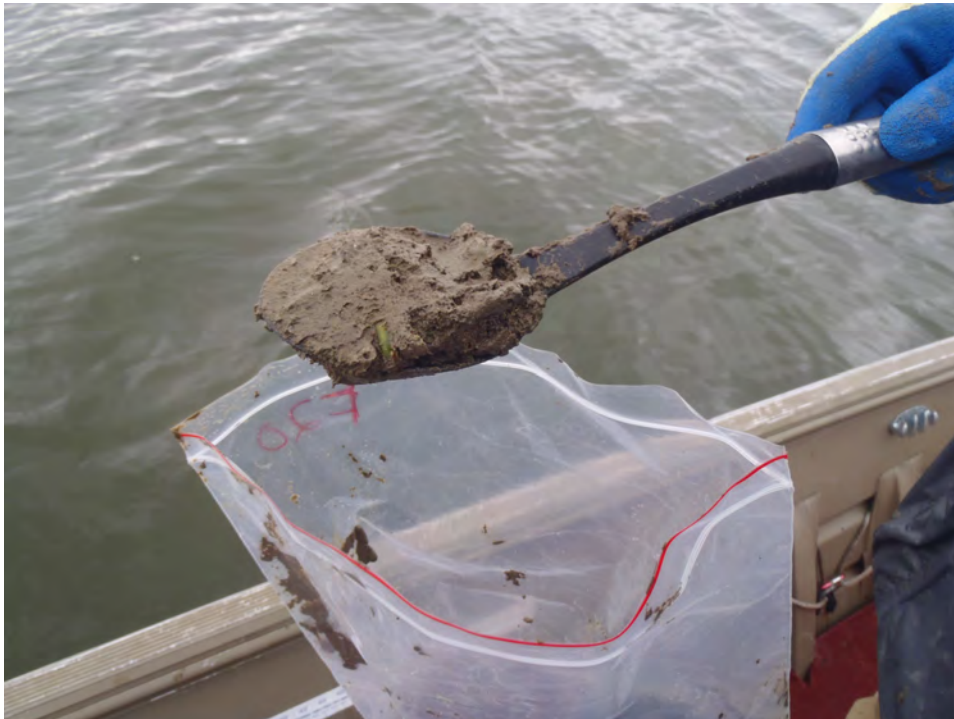
Figure 1. Lake Riley sediments in the growing zone varies from a mucky sediment to a silty-sand mixture. This picture shows a silty-sand sediment in Lake Riley.
