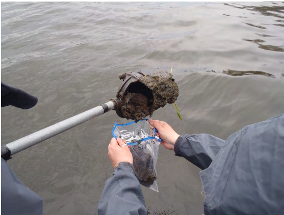
Figure S1. Lake Susan sediments in the growing zone varies from a mucky sediment to a silty-sand mixture. This picture shows a silty-sand sediment in Lake Susan.
