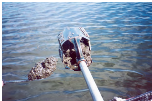
Figure 2a. Soil auger used to collect lake sediments in water depths to 7 feet.
