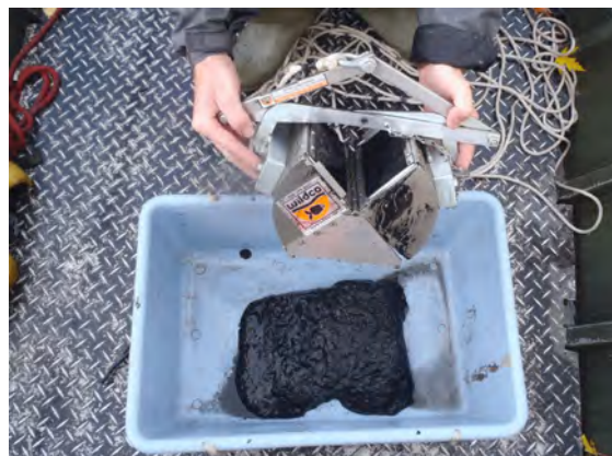
Figure 2b. Ponar dredge used to collect lake sediments in deeper water.
