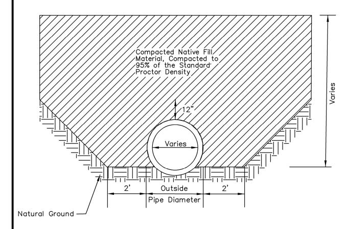
The bottom of the trench shall be shaped to fit the pipe barrel for at least 50% of the outside diameter
