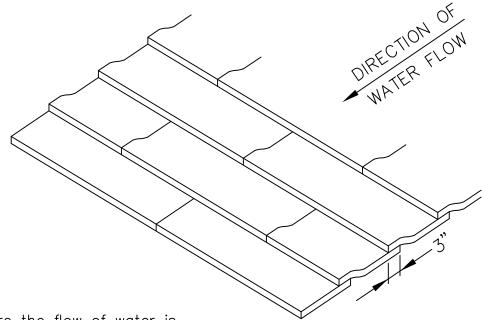
Where the flow of water is sheeting, place sod strips perpendicular to the direction of water flow.
