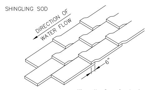
Where the flow of water is concentrated, place sod stips parallel to the direction of water flow.
