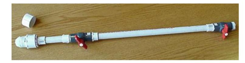
The wick applicator pictured here is designed for applying water-soluble herbicide products to cut stem surfaces. It can be assembled from commonly available PVC plumbing fittings and pipe. Starting at the top (right side of photo) and working down, the parts needed to build an applicator are:
